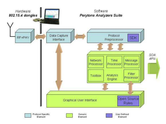
In addition to the graphical user interface, the user can add 'code like' elements to the analyzer, either by using the Peryton-Monitoring Add-On (with which he can create Open Source Rules and incorporate them into the analyzer environment) or through the Peryton-SDK Add-On that allows
