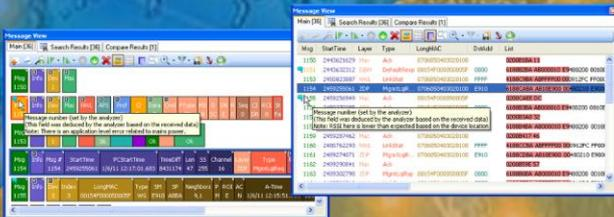
The Message Sequence View window shows the interaction between two and up to 8 devices in a single screen.
